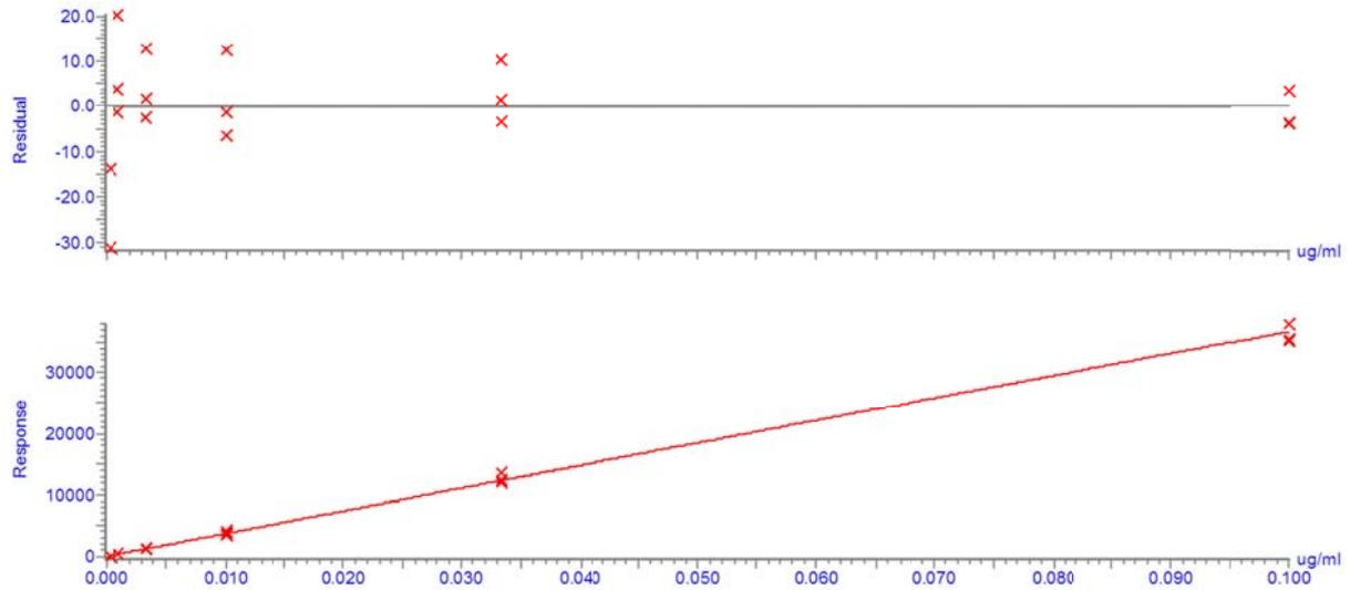
**Figure 3.** Examples of GC-MS/MS calibration curves for bifenazate matrix matched with maize for livestock feed (concentrations from 0.0003-0.1  $\mu\text{g/ml}$ )
