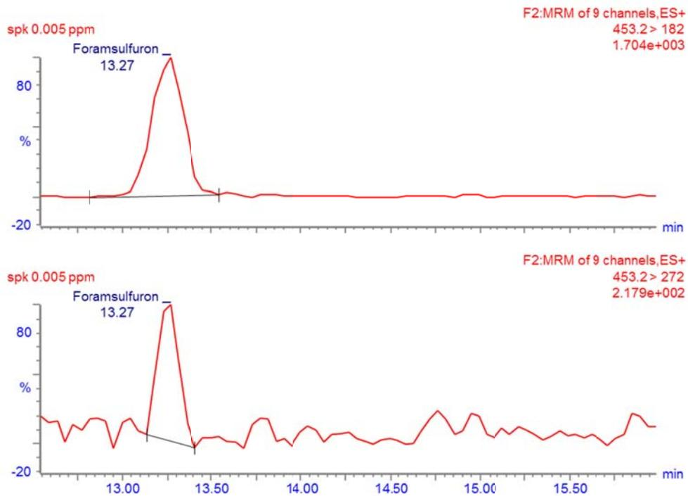
**Figure 2:** Examples of LC-MS/MS chromatograms foramsulfuron in maize for livestock feed obtained in positive mode when analysing extract spiked with 0.005 mg/kg (two MRM transitions are shown).
