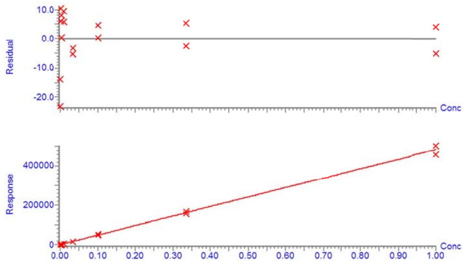
**Figure 4.** Examples of LC-MS/MS calibration curves for foramsulfuron matrix matched with maize for livestock feed (concentrations from 0.001-1.0  $\mu\text{g/ml}$ ).
